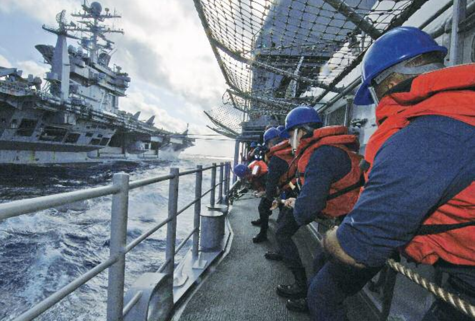
Sailors aboard USS Monterey heave the fuel line during a fuel at sea replenishment.
