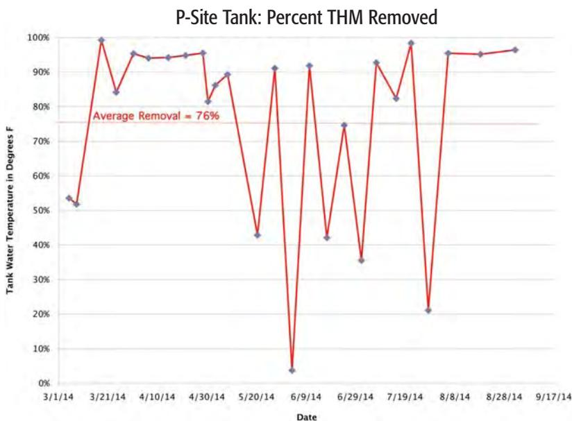
and THM concentrations were assessed as part of this initial test. Initial pilot test results were very promising. Over ten days, approximately 90 percent of the THM were removed from the tank water. Chlorine usage by the chlorine injection system did not increase, indicating that the chlorine in the water was not being stripped by the spray aeration system. In fact, it appeared that
