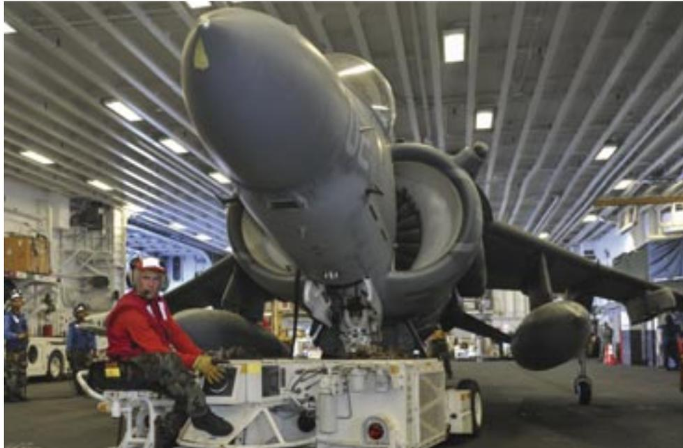
NESDI project 328 is testing and authorizing a trivalent chromium process as a non-chromated replacement. Post-treatment coatings are used widely on landing gear for the AV-8B and other aircraft.
