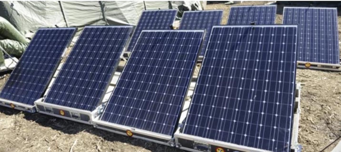
GREENS, one of five PORs for renewable energy systems, is a 300-watt photovoltaic battery system developed by ONR that can provide continuous power to Marines in the field.
