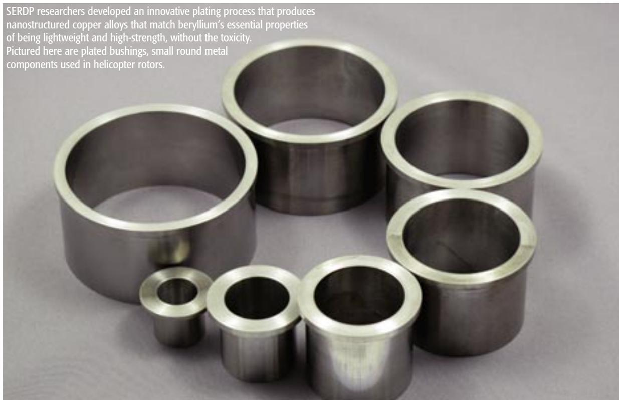
This project developed and validated a nanocrystalline copper electroplating process that produces an environmentally benign copper alloy that matches the desirable properties of copper-beryllium.
