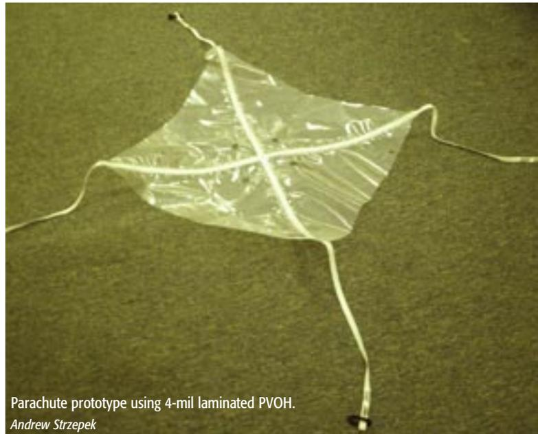
Parachute prototype using 4-mil laminated PVOH.
