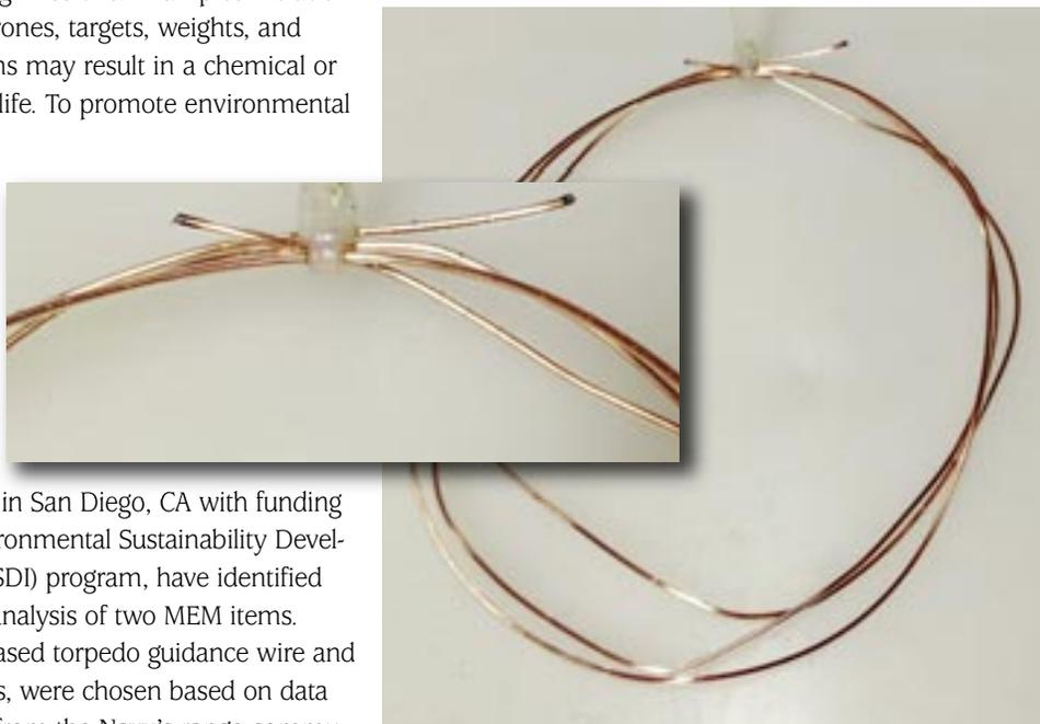
Copper torpedo guidance wire with plastic coating intact after 45 days.
