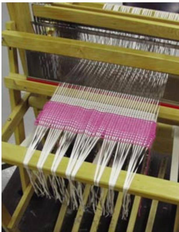
Weaving process for the new PVA parachute prototype.
