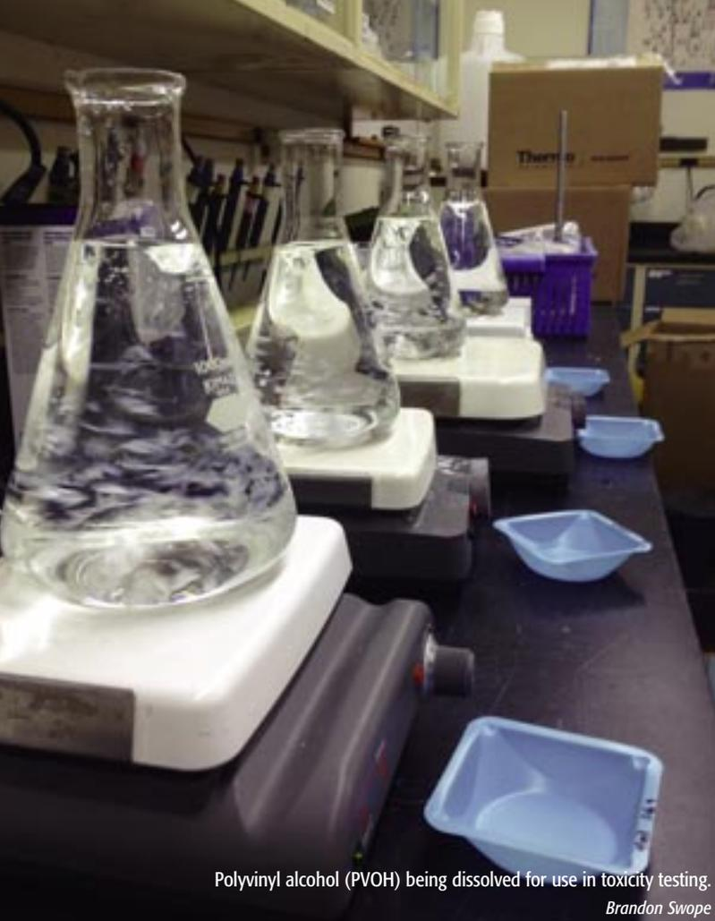
Polyvinyl alcohol (PVOH) being dissolved for use in toxicity testing.
