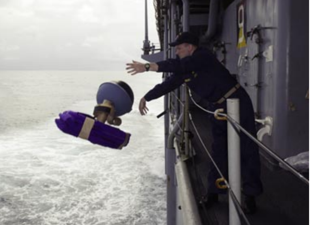
Jeffrey Grabon launches a global drifter buoy into the Pacific Ocean from the amphibious dock landing ship USS Pearl Harbor (LSD 52) while underway for Pacific Partnership 2013. The buoy, belonging to the Scripps Institution of Oceanography, is used to measure ocean currents up to 15 meters in depth, sea surface temperatures, and atmospheric pressure. Pacific Partnership is the largest disaster response-preparation mission in the Indo-Asia-Pacific region.
