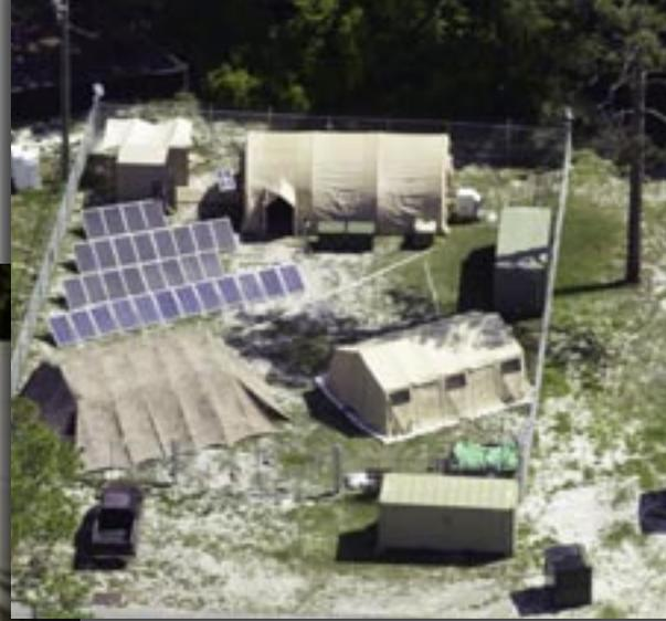
NSWC PCD's expeditionary energy compound runs completely on solar power and uses fossil fuels as needed. A commercial-off-the-shelf water fountain offers researchers potable water captured from moisture in the air. Sensors are placed inside and outside the tents to capture radiant barrier and heat readings.
