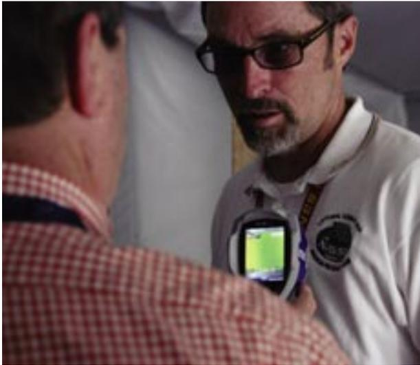
NSWC PCD engineers Bob Backus (left) and Ray Sheffield (right) use a handheld thermal imaging device to determine heat levels inside a tent being used for energy absorption and monitoring research conducted at NSWC PCD.
