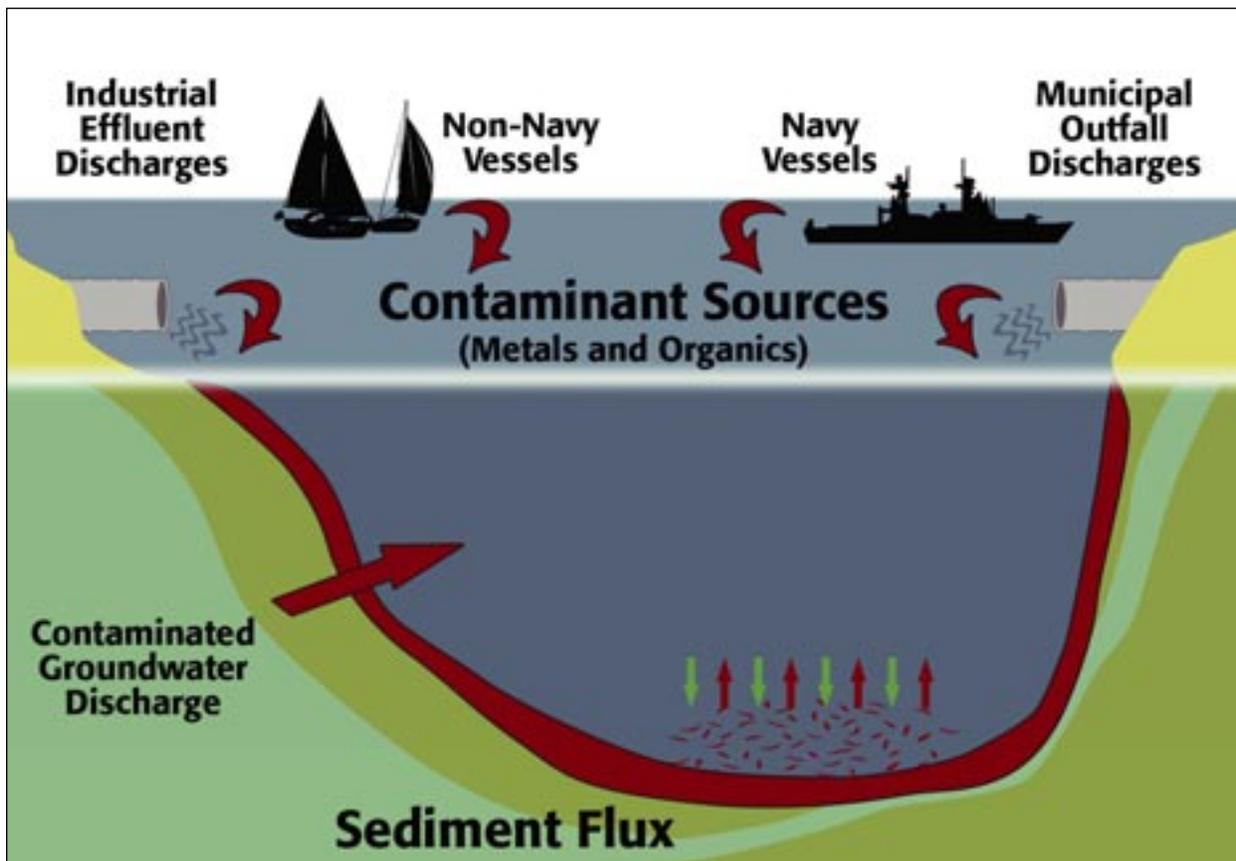
Examples of point and non-point sources of copper in San Diego Bay, CA. Point sources are those with well-defined physical discharges, while non-point sources are not physically well defined. In this figure, non-point sources include runoff from urbanized/industrialized areas, both civil and military.
