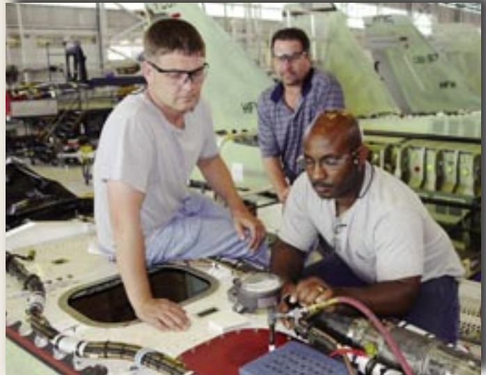
Aircraft Mechanic Patrick Dodrill (from left), Mechanical Systems Engineer Patrick Papay, and Darvin Etienne monitor a pressure decay test to detect the presence of a fuel leak on an F/A-18 Green Hornet Strike Fighter aircraft at FRCSE.
