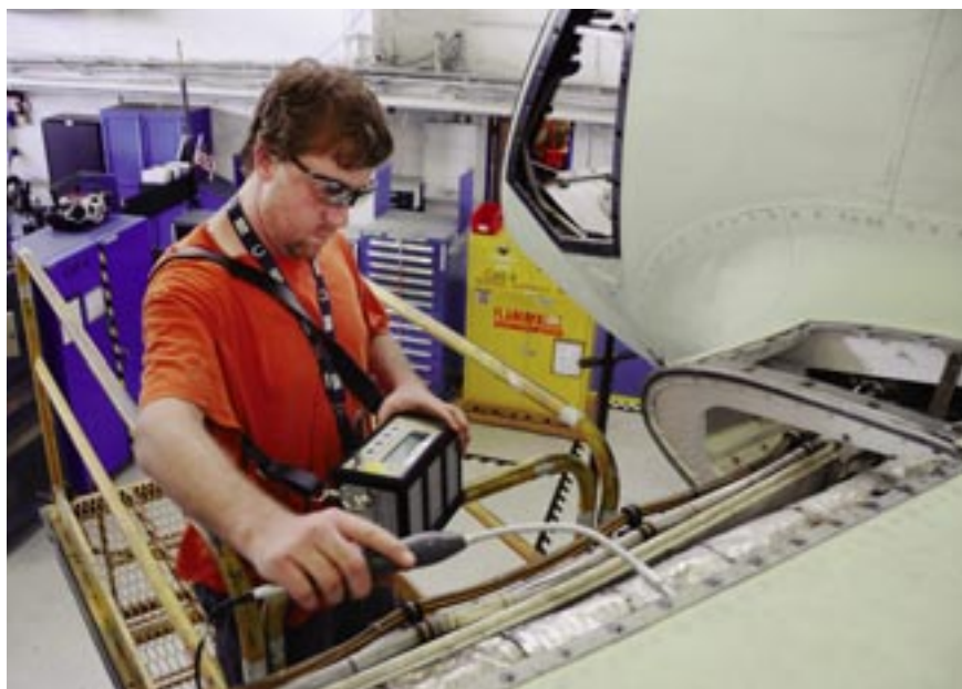
Sheet Metal Mechanic Bryan Swafford inspects a P-3 Orion wing tank for potential fuel leaks using hydrogen leak detection technology at FRCSE. This new capability has reduced the TAT of aircraft wet check by 15 percent.
