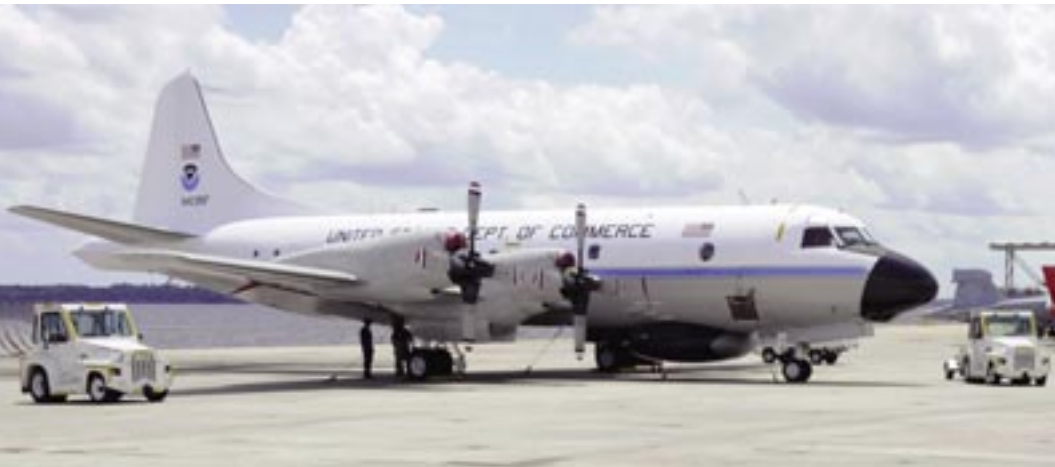
A WP-3D aircraft operated by the National Oceanic and Atmospheric Administration's Aircraft Operations Center sits on the airfield at FRCSE as maintainers perform a visual inspection. The aircraft is one of two hurricane hunters used for long-range atmospheric research. They are civilian versions of the U.S. Navy's P-3 four-engine maritime reconnaissance aircraft and are maintained and repaired at FRCSE on Naval Air Station Jacksonville, Florida.
