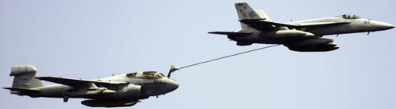
An EA-6B Prowler and an F/A-18E Super Hornet perform a refueling exercise during an air power demonstration aboard the aircraft carrier USS John C. Stennis (CVN 74).
