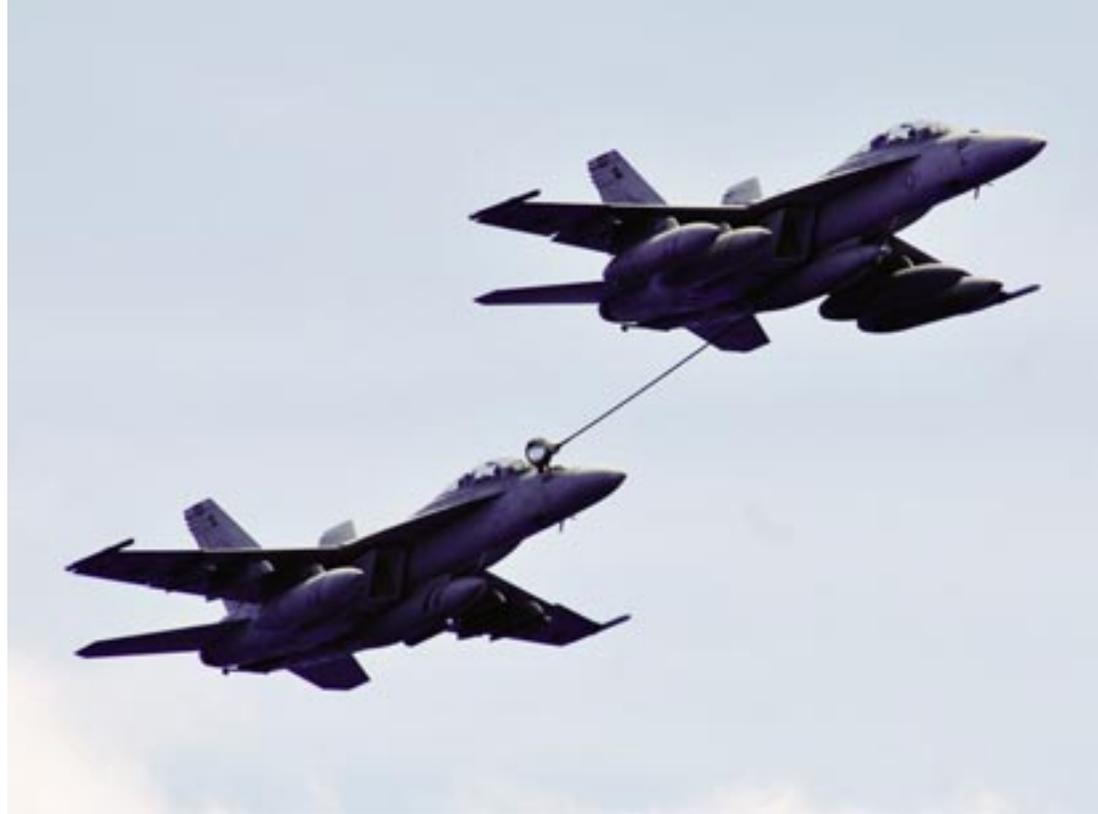
F/A-18F Super Hornets perform the SMART refueling practice that saves energy by configuring a Super Hornet tanker with only the centerline refueling tank. The tanker launches to refuel the aircraft returning from their mission then lands within about 20 minutes. Referred to as “Yo-yo Tanking” in the fleet, this method delivers up to 5,000 pounds of fuel per tanker without incurring undue drag, weight or efficiency penalties.
