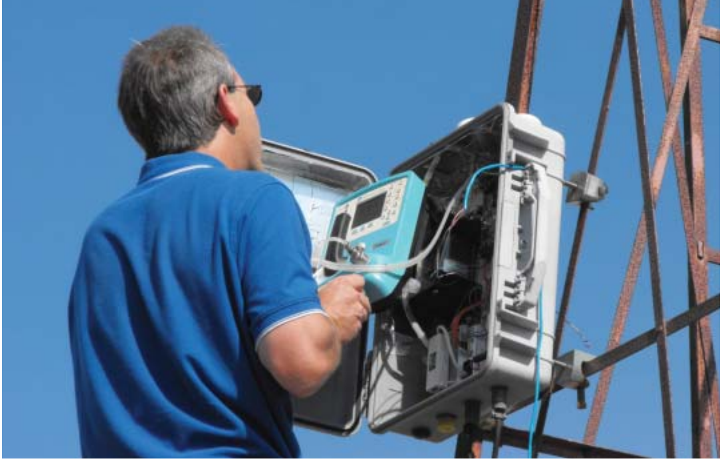
Sonic boom monitors, like this one installed and calibrated at Pax River, are an important part of the base's initiative to limit noise disturbances.
