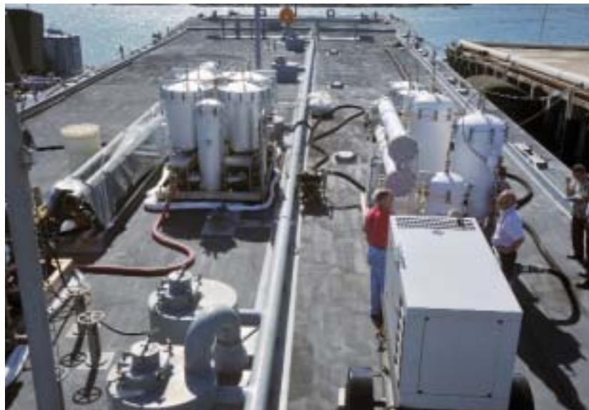
Pearl Harbor's new fuel and comp water cleaning system consists of the fuel cleaner subsystem (at right behind the generator), the comp water cleaner (at left center) and the zinc remover (at far left).
