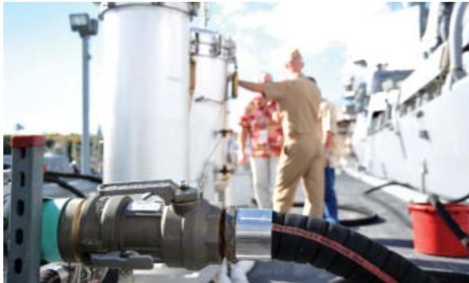
A no-drip hose connection between a fuel barge and USS Chung-Hoon.
