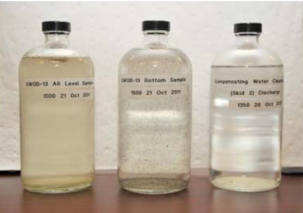
Left and center, samples of comp water from two levels in the holding tank of a ship waste off-loading barge (SWOB). At right, water from the same tank after being run through the comp water cleaner.
