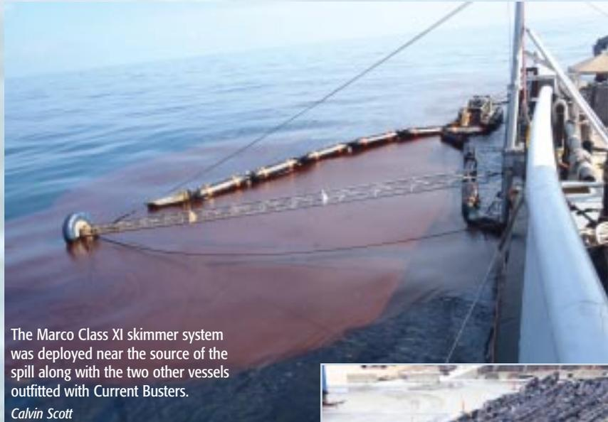
The Marco Class XI skimmer system was deployed near the source of the spill along with the two other vessels outfitted with Current Busters.
