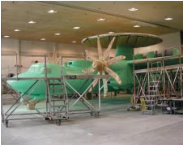
This E-2C was the first such aircraft to have the entire exterior of the aircraft primed with Deft's non-chrome primer.
