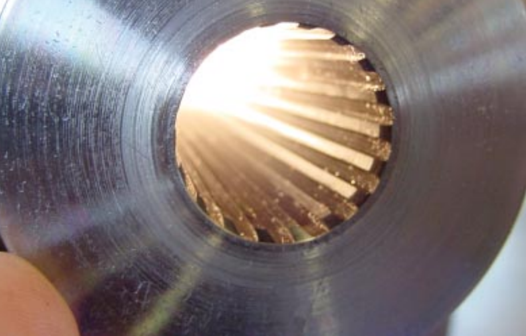
SERDP's Weapons Systems and Platforms Project of the Year, led by Mr. Mark Miller, developed a method for applying an environmentally benign tantalum-tungsten coating onto the interior surfaces of medium caliber gun barrels. Gun barrels coated with tantalum-tungsten last three times as long as barrels coated with hazardous hexavalent chromium.
