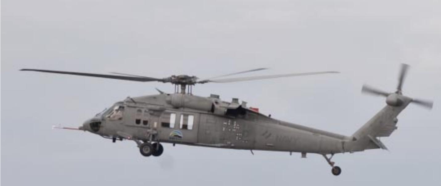
A U.S. Navy MH-60S Sea Hawk helicopter assigned to the Blackjacks of Air Test and Evaluation Squadron (HX) 21 tests a 50/50 camelina seed-based biofuel blend at NAS Patuxent River, MD. The test demonstrates another step toward the certification of fuels from non-petroleum sources for use in all Navy and Marine Corps aircraft.
