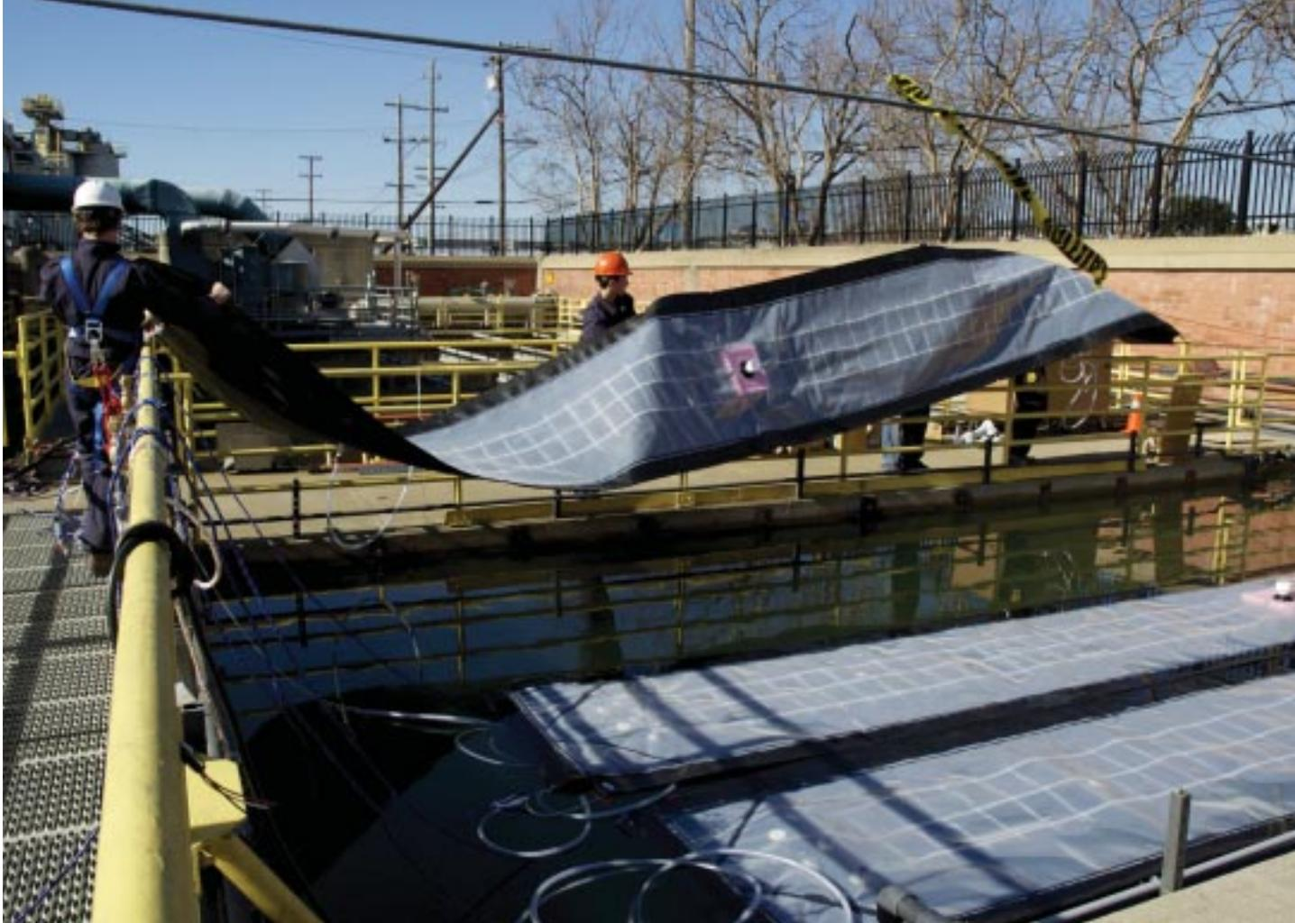
Prototype OMEGA photobioreactors being deployed in seawater tanks to grow microalgae on wastewater from the nearby sewage treatment plant.
