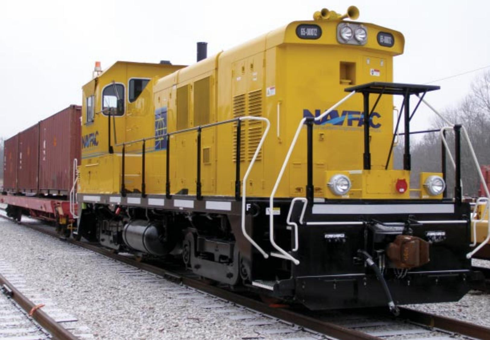
A new environmentally-friendly 120-ton switcher locomotive, the N-ViroMotive, pulls ordnance cars at NSA Crane. It is one of eight locomotives used on base to stage CAAA ordnance for shipment to U.S. forces around the world. Procured and operated by NAVFAC Midwest's PWD Crane, it runs on bio-diesel fuel and is certified by EPA for low emissions.
