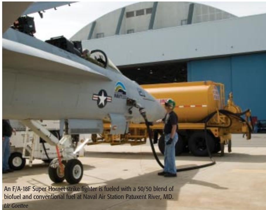
An F/A-18F Super Hornet strike fighter is fueled with a 50/50 blend of biofuel and conventional fuel at Naval Air Station Patuxent River, MD.
