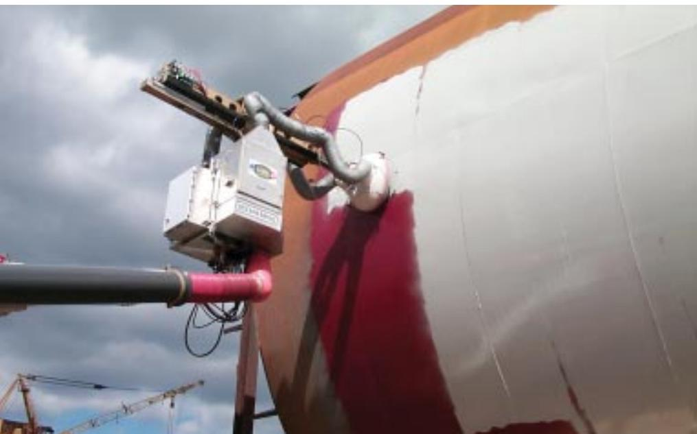
APACTS, a predecessor of the MAEE, was designed to be an automated system using an integrated dome-covered nozzle and vacuum technology to help minimize overspray at its source.
