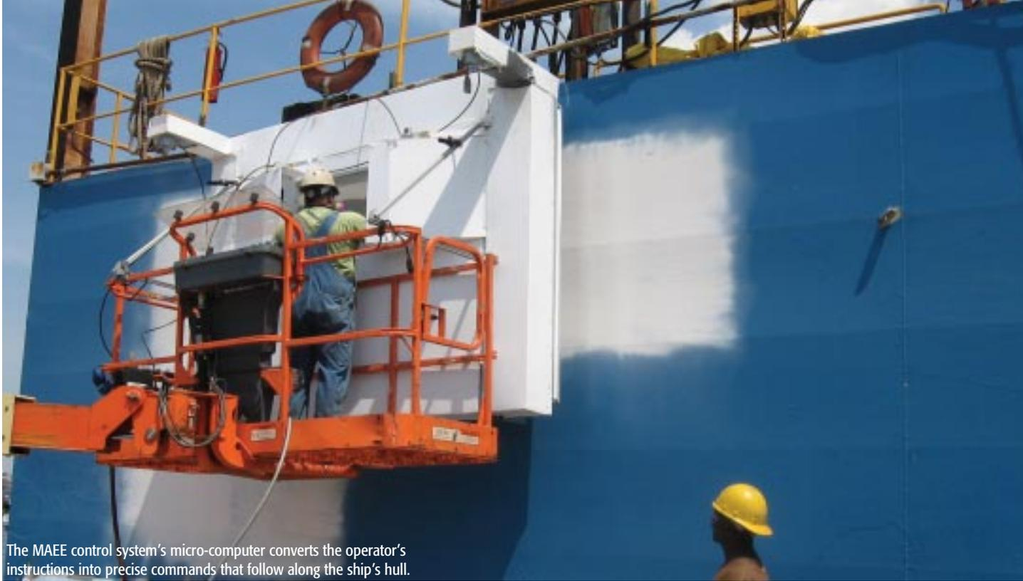
The MAEE control system's micro-computer converts the operator's instructions into precise commands that follow along the ship's hull.
