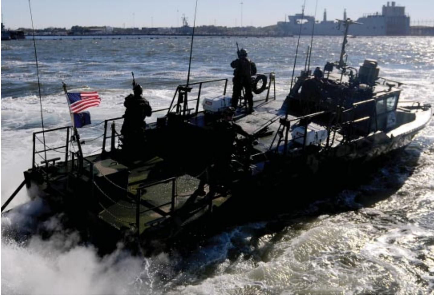
On 22 October 2010, the Navy conducted a full power demonstration of this alternative fuel-powered RCB-X running on a blend of 50 percent algae-based and 50 percent petroleum-based fuel, achieving a speed topping 44 knots (about 52 miles per hour).
