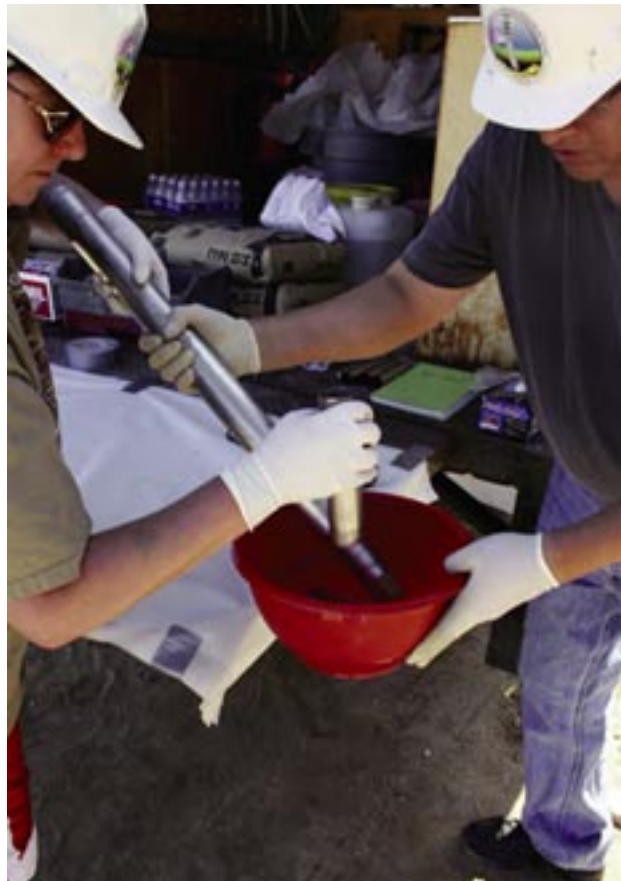
Edward's Site 285 soil samples as deep as five meters below ground level were collected for later analysis using EPA Standard Method 6860.
